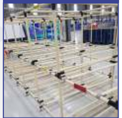
(J-4) SLIDING PIPE FIFO RACK
